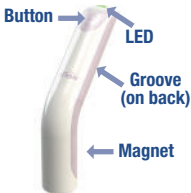
Figure 12. Activator button, LED light and magnet positions
