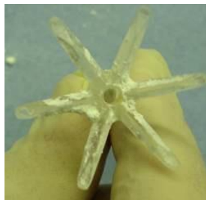
Figure 8b. The inFlow device post-study, showing minimal encrustation and a clear central lumen after 9 days of draining bacteria-saturated urine substitute
