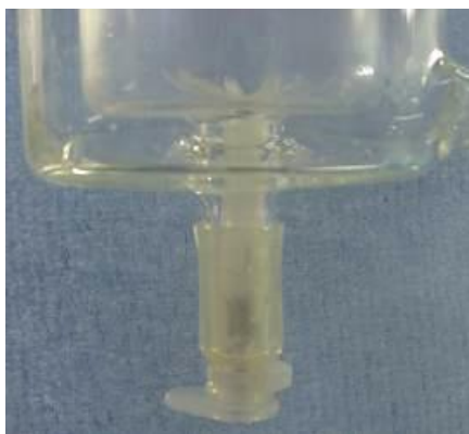
Figure 8a. The inFlow device during study, shown in place in the outlet of bladder model
